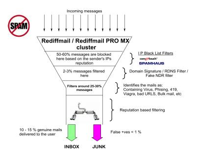
We use a combination of both the techniques to filter out unwanted mails and keeps the users mailbox free from spam. Different modules in the Rediffmail enterprise spam control system are IP based filtering, Domain Signatures / RDNS and Fake NDR filters, Content based filtering, and Reputation based filtering.
