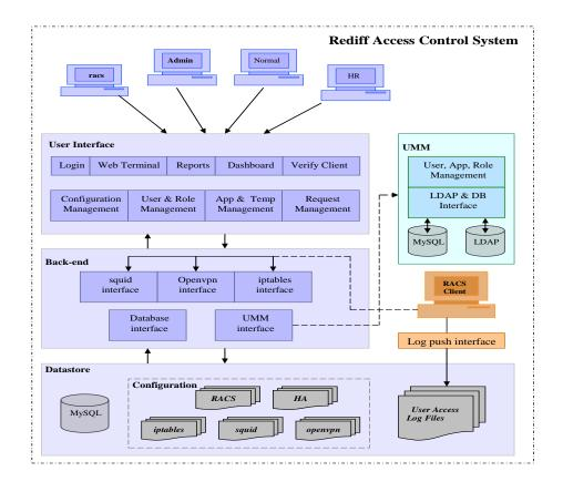
The Application also contains a User Management facility to effectively manage users of the system and a local database for effective data management. It has three main components
